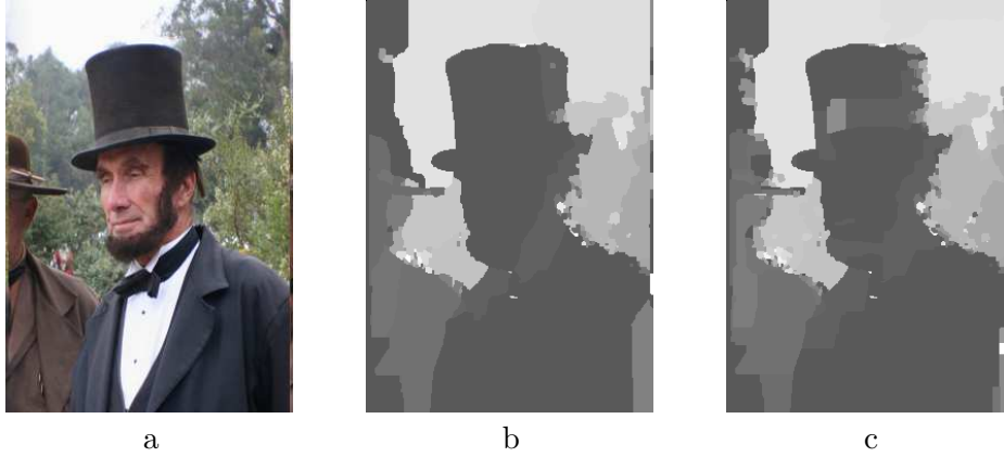
Figure 1.1 a. A single frame from a stereo pair. Finding the disparity is often done by minimizing an energy function. b. The results of graph cuts using a Potts model energy function. c. The results of ordinary BP using the same energy function.
