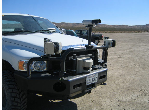
Figure 2. The Golem/UCLA group vehicle used as our test platform. In this installation the camera is mounted inside a housing on top of a pole connected to the front bumper. Other installations had the camera mounted on the windshield.
