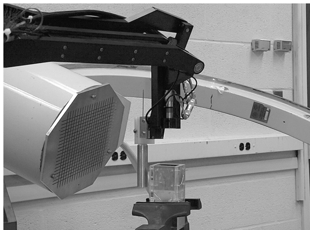
Figure 8. Experimental setup at The Johns Hopkins University for image-guided positioning showing the C-arm with the dewarping grid plate mounted on its image intensifier (left), the LARS robot arm holding the probe (center top) and a box (center bottom).
