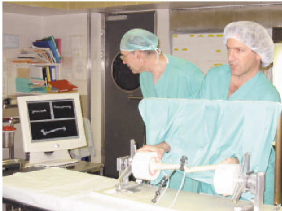
Fig. 6. Experimental setup for fracture reduction based on periaxial rotation values. The surgeon on the right manipulates the fragments without seeing them according to the indications of the surgeon on the left, who can see the bone-fragment models and periaxial rotation value on the screen.
