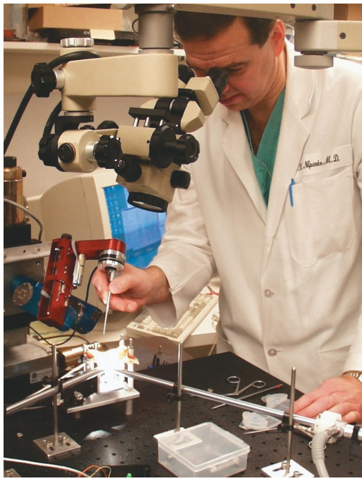
Figure 7. The Steady Hand microsurgical-assistant robot.
