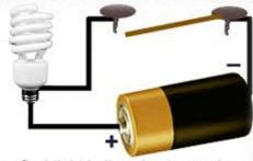
Use a flashlight bulb and not a regular light bulb when doing the experiment.
