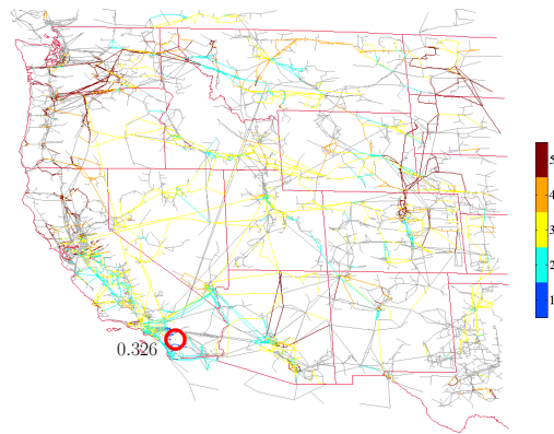
Fig. 2. Simulation of a geographically correlated failure in the San Diego area. All power lines, power plants, and substations within the marked 50 km radius disk were removed at round 1. The colors represent the rounds in which additional lines faulted. The final yield (the fraction of the original demand that was satisfied at the end of the cascade) is 0.326.
